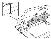
Install the USB driver. Refer to Installation Manual on the CD-ROM included with KX-DT301. Attach the KX-DT301 to your unit with the screws (included with KX-DT301).
