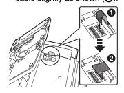
Attach the KX-NT303 to your unit with the screws (included with KX-NT303).
